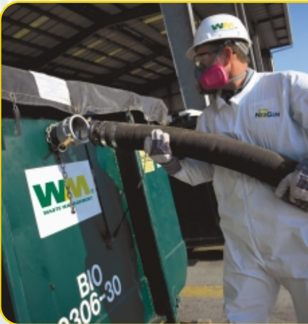
Conducted under controlled conditions, BioSite SM bioremediation uses a combination of chemicals and microorganisms to naturally break down hazardous materials into non-hazardous substances that can be recycled or buried in conventional landfills.
