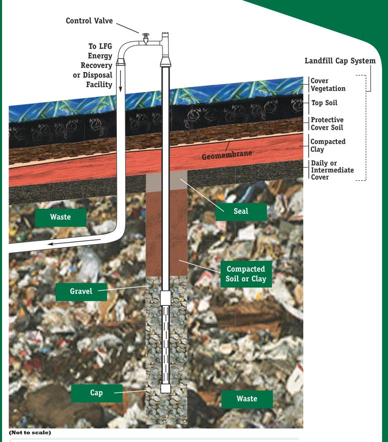
Gas extraction wells are used to collect gas that is generated as the waste decomposes. The gas is used to produce energy or is sent to a landfill gas disposal facility.
