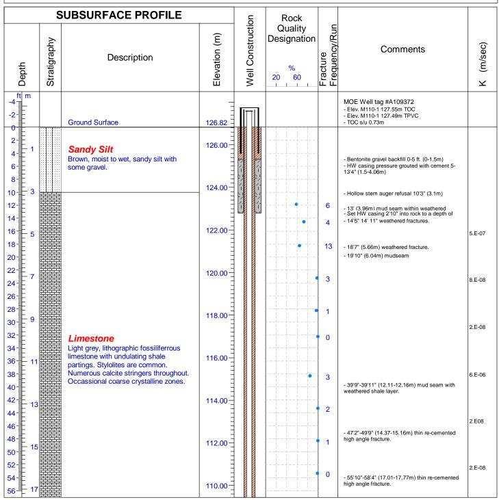
Drilled By: Aardvark Drilling Inc. Drill Method: Diamond Drilling Hole Size: HQ3 3.78 (96mm) Drill Date: February 7-9, 2011
