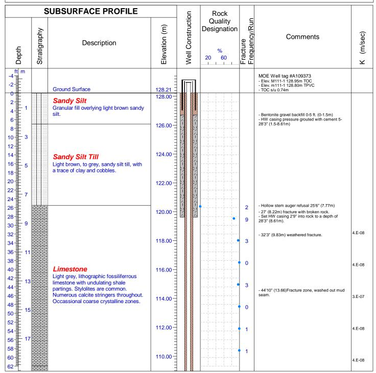
Drilled By: Aardvark Drilling Inc. Drill Method: Diamond Drilling Hole Size: HQ3 3.78 (96mm) Drill Date: February 9,10, 2011 Drill Angle: Vertical Azimuth: n.a. Datum: NAD 83 Zone 18 Checked By: P.T.
