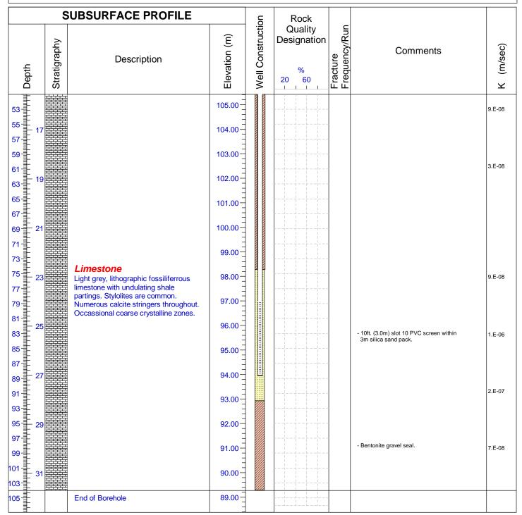
Drilled By: Aardvark Drilling Inc. Drill Method: Rotary Tri-cone Hole Size: 3.78" (96mm) Drill Date: May 17, 2012 Drill Angle: Vertical Azimuth: n.a. Datum: NAD 83 Zone 18 Checked By: P.T.
