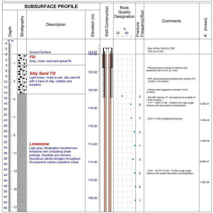
Drilled By: Aardvark Drilling Inc. Drill Method: Diamond Drilling Hole Size: HQ3 3.78" (96mm) Drill Date: August 16, 17, 2010 Drill Angle: Vertical Azimuth: n.a. Datum: NAD 83 Zone 18 Checked By: D.H.
