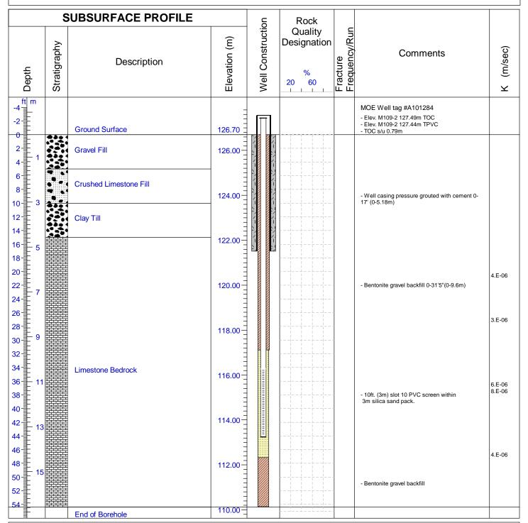
Drilled By: Chalk Well Drilling Ltd.
