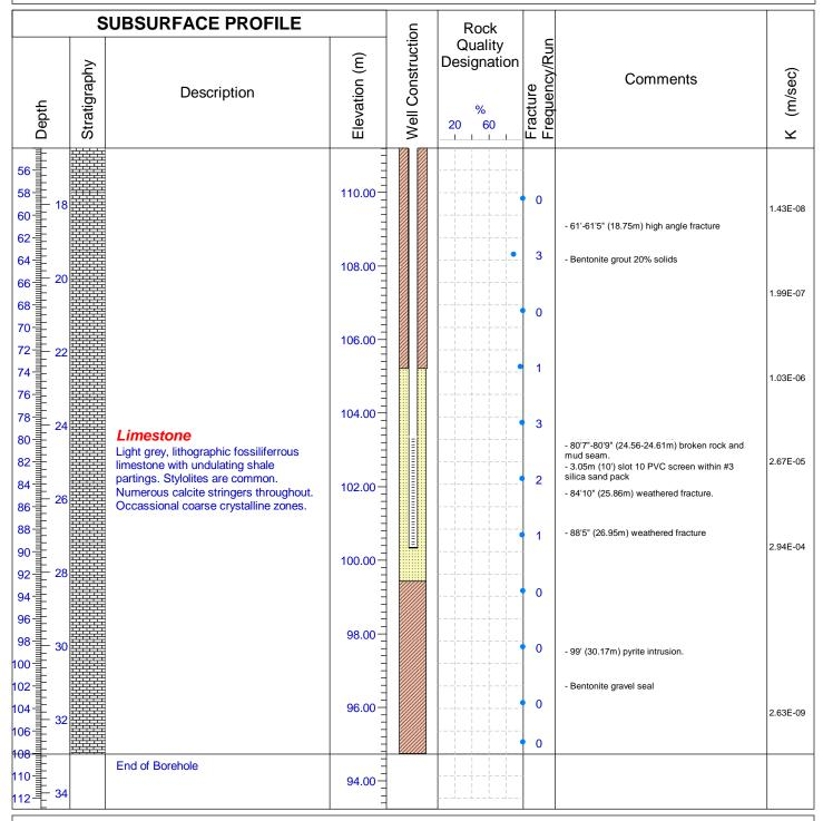
Drilled By: Aardvark Drilling Inc. Drill Method: Diamond Drilling Hole Size: HQ3 3.78" (96mm) Drill Date: August 19, 20, 2010
