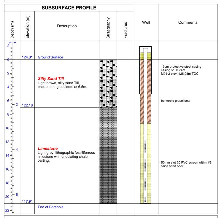
Drilled By: MPI Drilling Ltd. Drill Method: Air Hammer Drill Date: Oct.24, 2006 Hole Size: 10cm/4" Datum: m.a.s.l. Checked by: FAR
