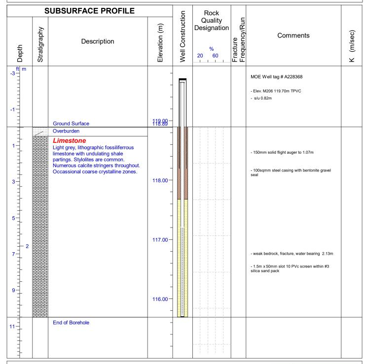
Drilled By: GET Drilling Ltd.
