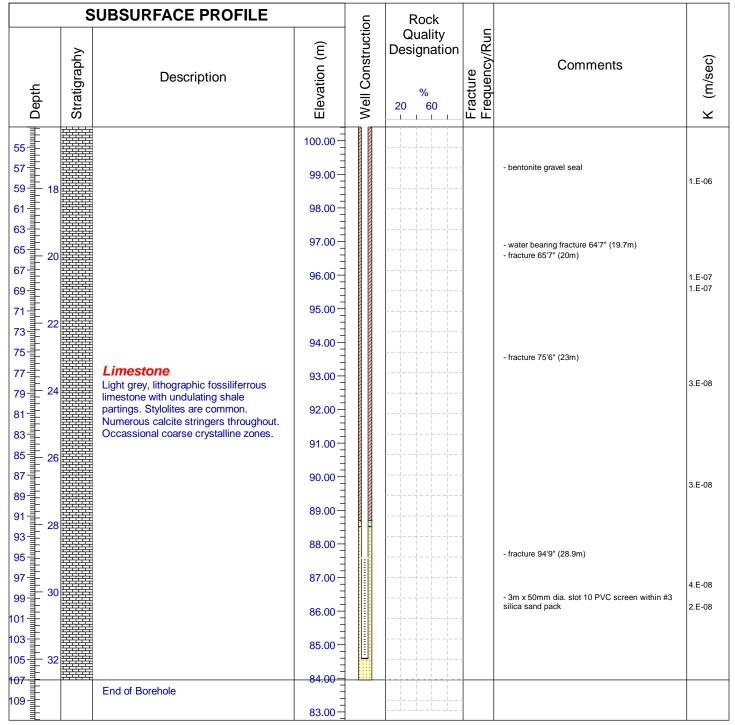
Drilled By: GET Drilling Ltd. Drill Method: Rotary Tri-cone Hole Size: 3.87" (98mm) Drill Date: June 17, 18, 2014 Drill Angle: Vertical Azimuth: n.a.
