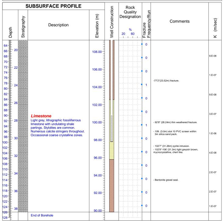
Drilled By: Aardvark Drilling Inc. Drill Method: Diamond Drilling Hole Size: HQ3 3.78 (96mm) Drill Date: February 9,10, 2011
