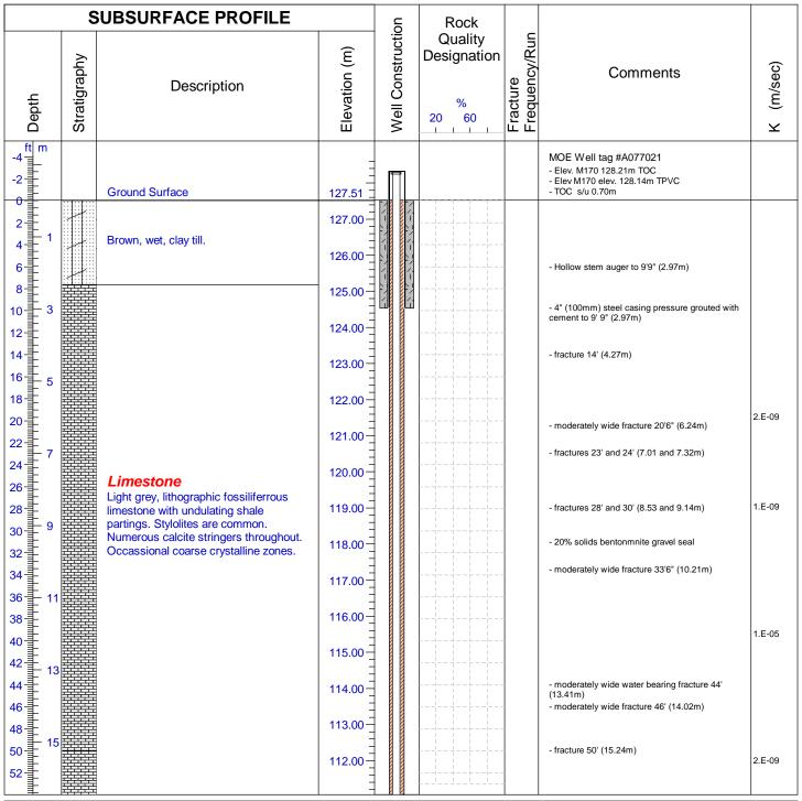
Drilled By: GET Drilling Ltd. Drill Method: Rotary Tri-cone Hole Size: 3.87" (98mm) Drill Date: March 7, 14, 2013 Drill Angle: Vertical Azimuth: n.a. Datum: NAD 83 Zone 18 Checked By: P.T.
