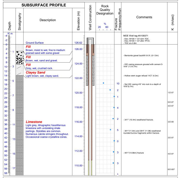
Drilled By: Aardvark Drilling Inc. Drill Method: Diamond Drilling Hole Size: HQ3 3.78 (96mm) Drill Date: February 3,4,7, 2011
