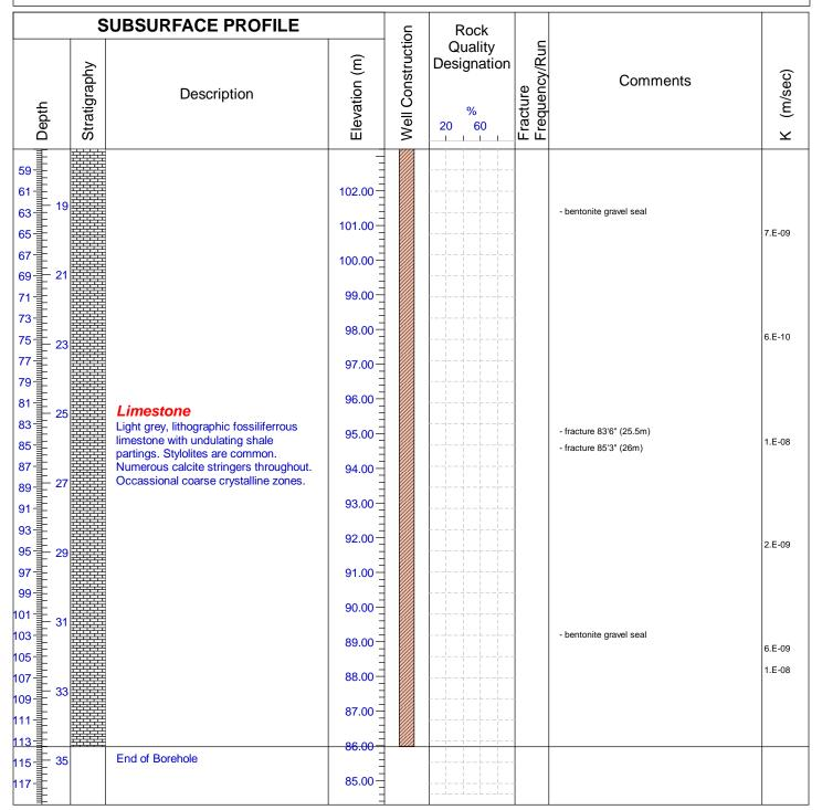
Drilled By: GET Drilling Ltd. Drill Method: Rotary Tri-cone Hole Size: 3.87" (98mm) Drill Date: June 17, 19, 2014 Drill Angle: Vertical Azimuth: n.a.
