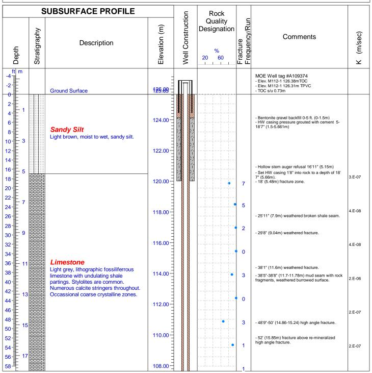
Drilled By: Aardvark Drilling Inc. Drill Method: Diamond Drilling Hole Size: HQ3 3.78 (96mm) Drill Date: February 11, 14, 2011
