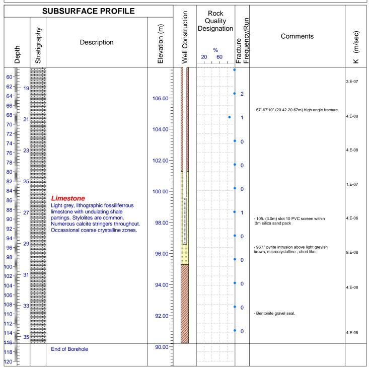
Drilled By: Aardvark Drilling Inc. Drill Method: Diamond Drilling Hole Size: HQ3 3.78 (96mm) Drill Date: February 11, 14, 2011 Drill Angle: Vertical Azimuth: n.a. Datum: NAD 83 Zone 18 Checked By: P.T.
