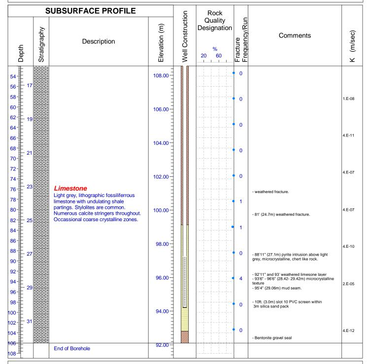
Drilled By: Aardvark Drilling Inc. Drill Method: Diamond Drilling Hole Size: HQ3 3.78 (96mm) Drill Date: February 23, 24, 2011 Drill Angle: Vertical Azimuth: n.a. Datum: NAD 83 Zone 18 Checked By: P.T.
