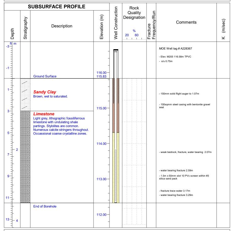
Drilled By: GET Drilling Ltd. Drill Method: Rotary Air Hammer Hole Size: 5" (127mm) Drill Date: April 17, 2018
