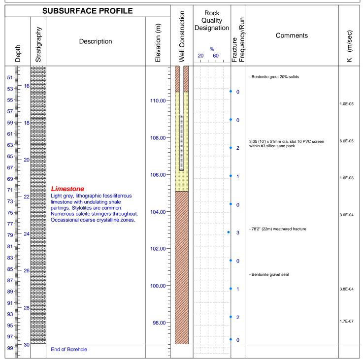
Drilled By: Aardvark Drilling Inc. Drill Method: Diamond Drilling Hole Size: HQ3 3.78" (96mm) Drill Date: March 30,31, 2009 Drill Angle: Vertical (90) Azimuth: n.a. Datum: NAD 83 Zone 18A Checked By: D.H.
