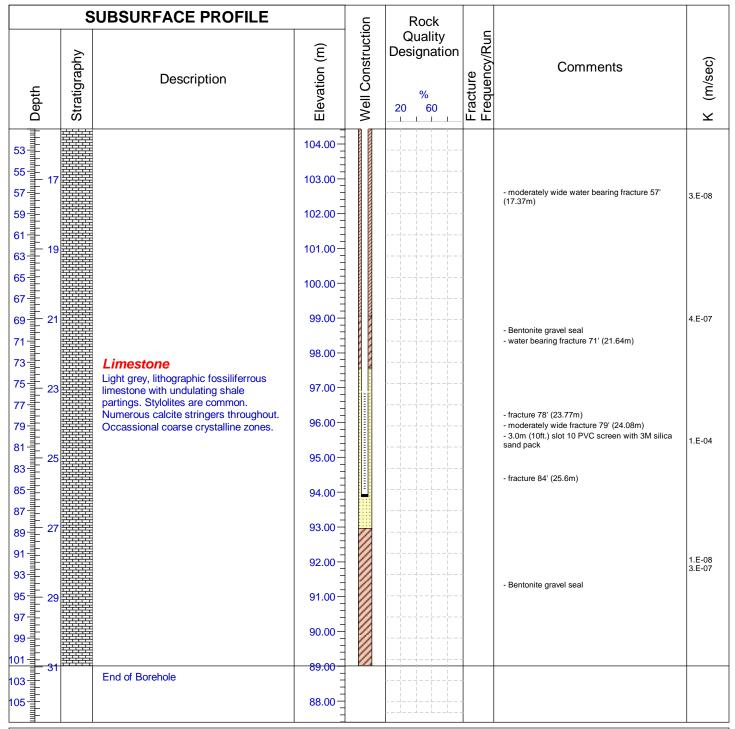
Drilled By: GET Drilling Ltd. Drill Method: Rotary Tri-cone Hole Size: 3.87" (98mm) Drill Date: March 6, 11, 2013 Drill Angle: Vertical Azimuth: n.a. Datum: NAD 83 Zone 18 Checked By: P.T.
