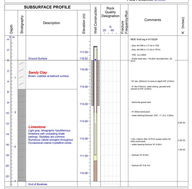
Drilled By: Aardvark Drilling Ltd. Drill Method: Rotary Tri-cone Hole Size: 6" (152mm) Drill Date: Aug. 15,17, 2015 Drill Angle: Vertical Azimuth: n.a. Datum: NAD83 Checked By: P.T.
