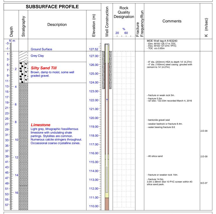
Drilled By: GET Drilling Ltd. Drill Method: Rotary Tri-cone Hole Size: 3.87" (98mm)
