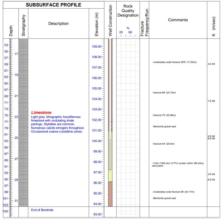
Drilled By: GET Drilling Ltd. Drill Method: Rotary Tri-cone Hole Size: 3.87" (98mm) Drill Date: March 6, 12, 2013 Drill Angle: Vertical Azimuth: n.a. Datum: NAD 83 Zone 18 Checked By: P.T.
