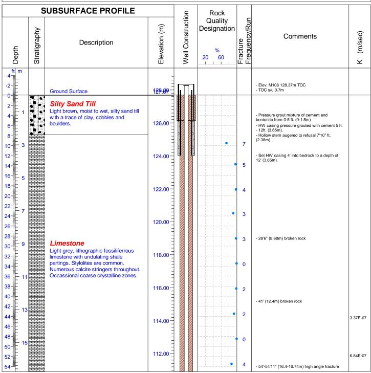
Drilled By: Aardvark Drilling Inc. Drill Method: Diamond Drilling Hole Size: HQ3 3.78" (96mm) Drill Date: August 19, 20, 2010 Drill Angle: Vertical Azimuth: n.a. Datum: NAD 83 Zone 18 Checked By: D.H.
