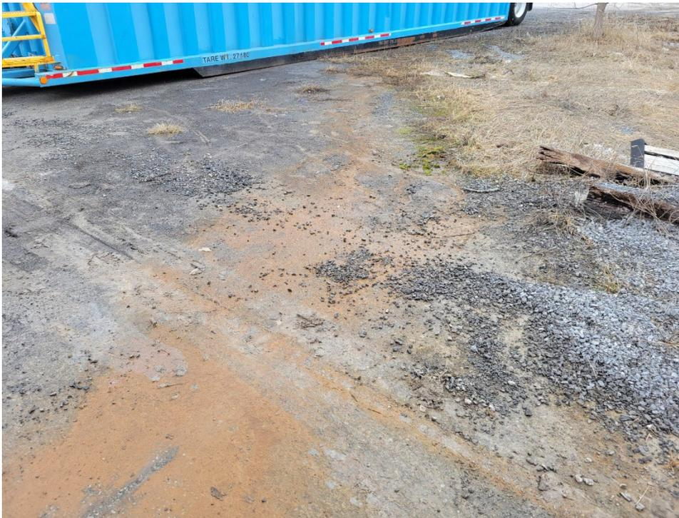
**Photo 2: Soil staining resulting from leachate released from leaking frac tank (March 27, 2023)**
