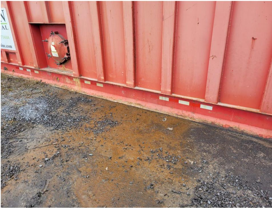
**Photo 1: Soil staining resulting from leachate released from leaking frac tank (March 27, 2023)**
