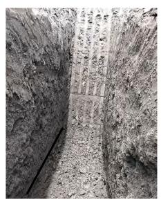
Photograph 2 – Compact Ablation Till to a depth of 11.5 feet at TP03-19.
