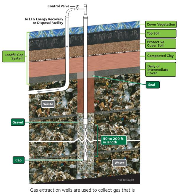
Gas extraction wells are used to collect gas that is generated as the waste decomposes. The gas is used to produce energy or is sent to a Landfill gas disposal facility.
