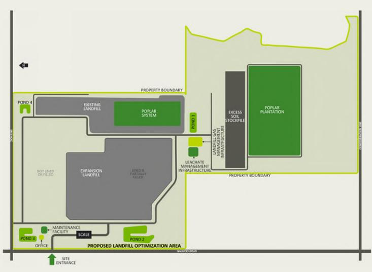
The purpose of the project is to provide additional landfill airspace of up to approximately 14M m<sup>3</sup> and extend site life by approximately 12 years (from 2031 to 2043).
