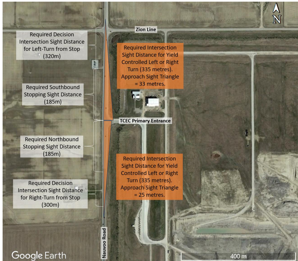
Figure 4-25. TCEC Primary Driveway Sight Distances
