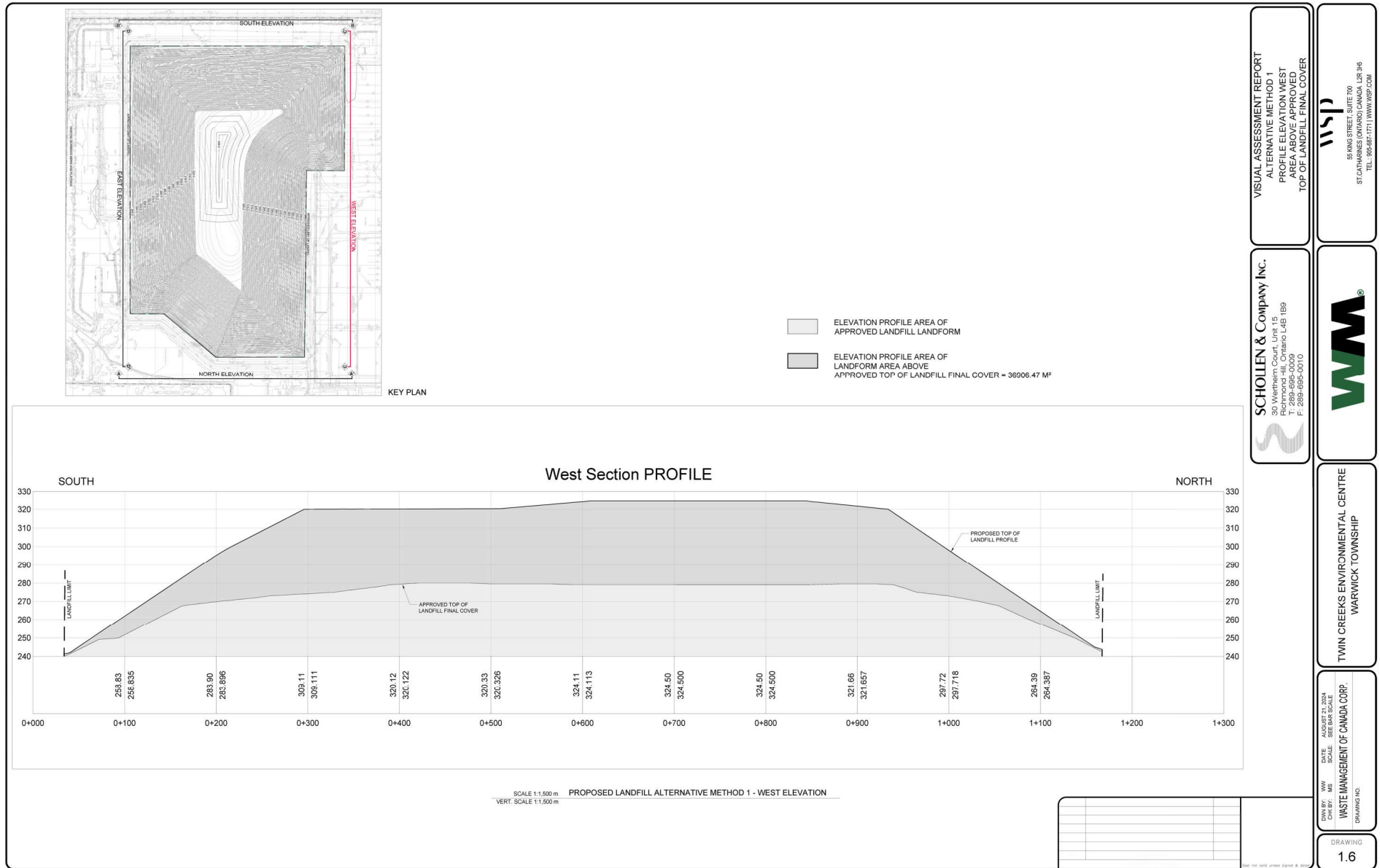
Figure 1-6. Alternate Method 1 – Profile Elevation West – Area Above Approved Top of Landfill Final Cover
