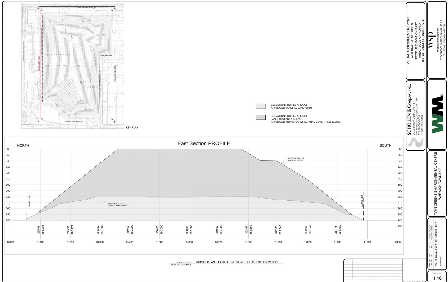
Figure 1-16. Alternate Method 3 – Profile Elevation East – Area Above Approved Top of Landfill Final Cover
