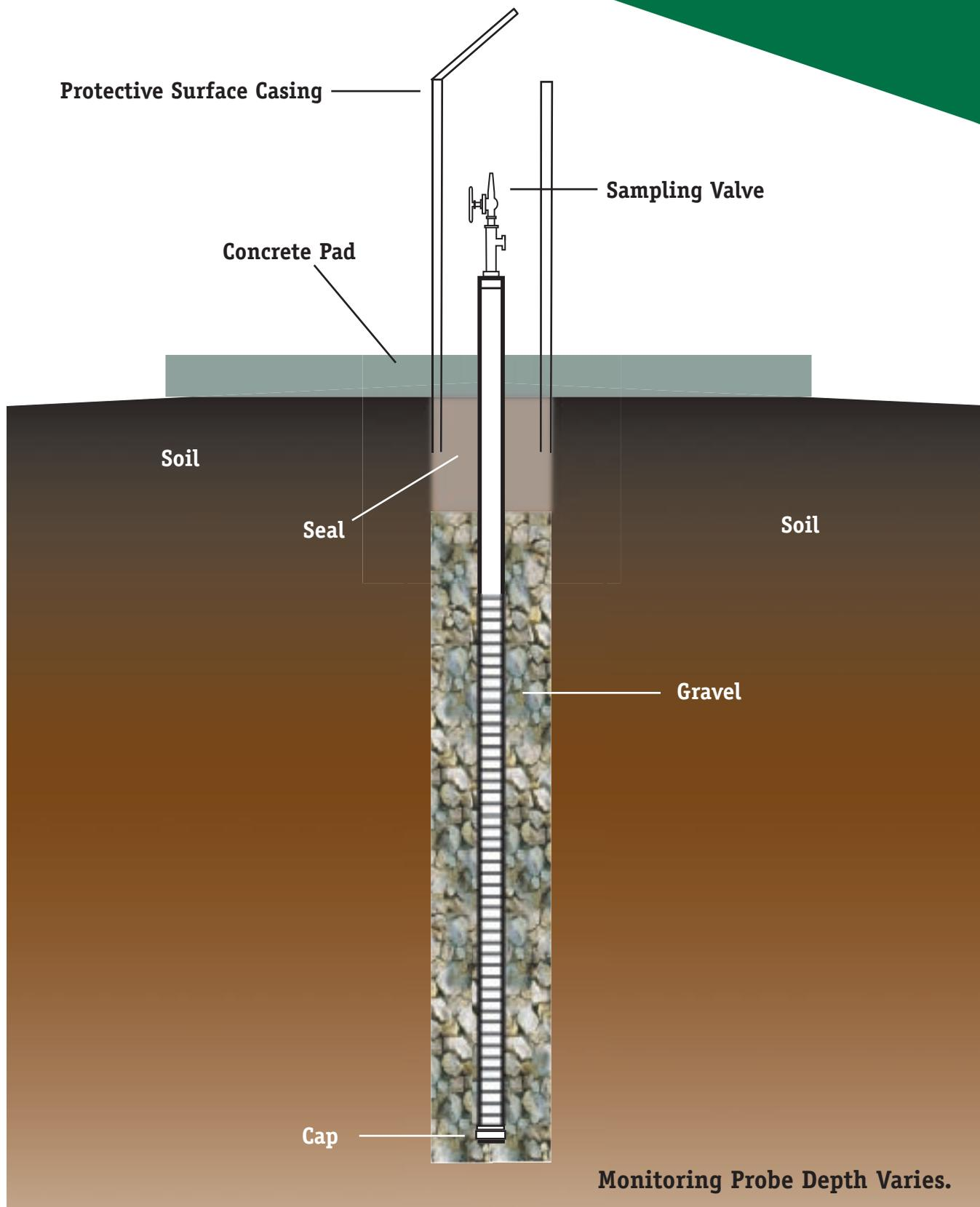
Gas monitoring probes are used to enhance environmental protection at landfills. Gas concentrations are measured at permit or regulatory specified time intervals. This process allows potential environmental concerns to be identified early, evaluated and corrected (when necessary) in accordance with regulations and sound scientific approaches.
