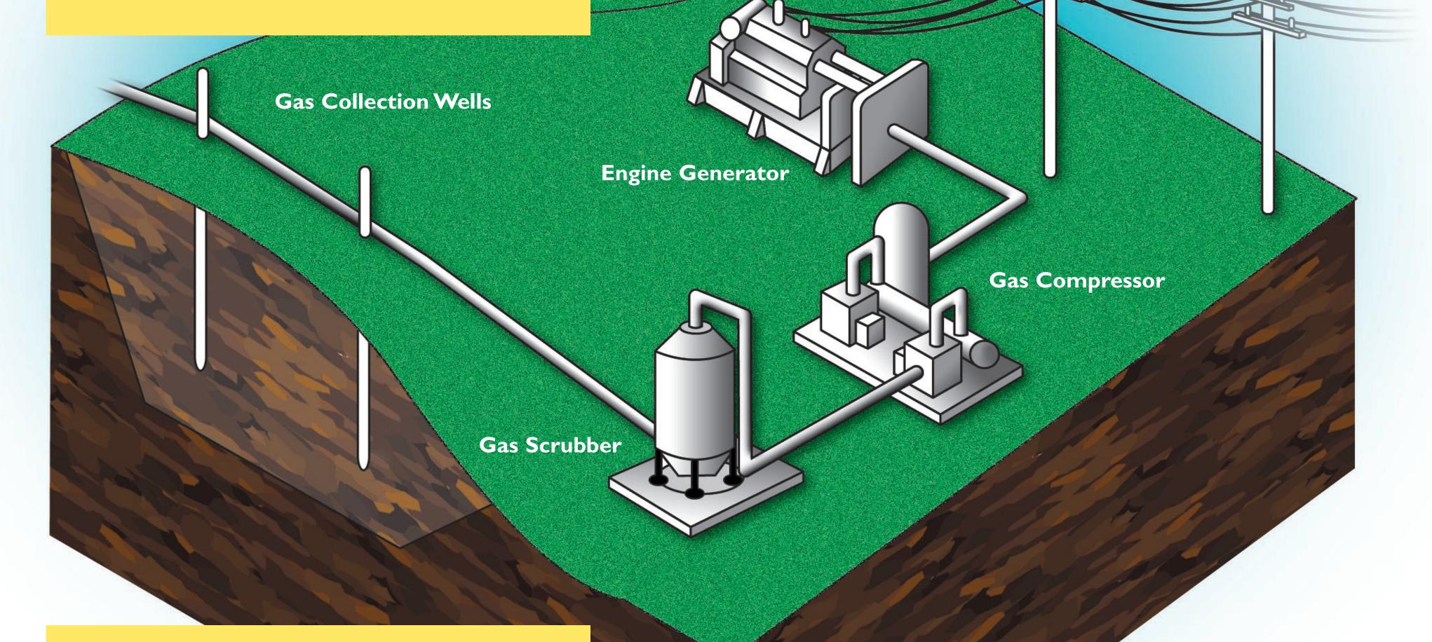
The methane gas is transported first to a gas scrubber, which extracts moisture and filters out particulates, and then to a compression facility.
