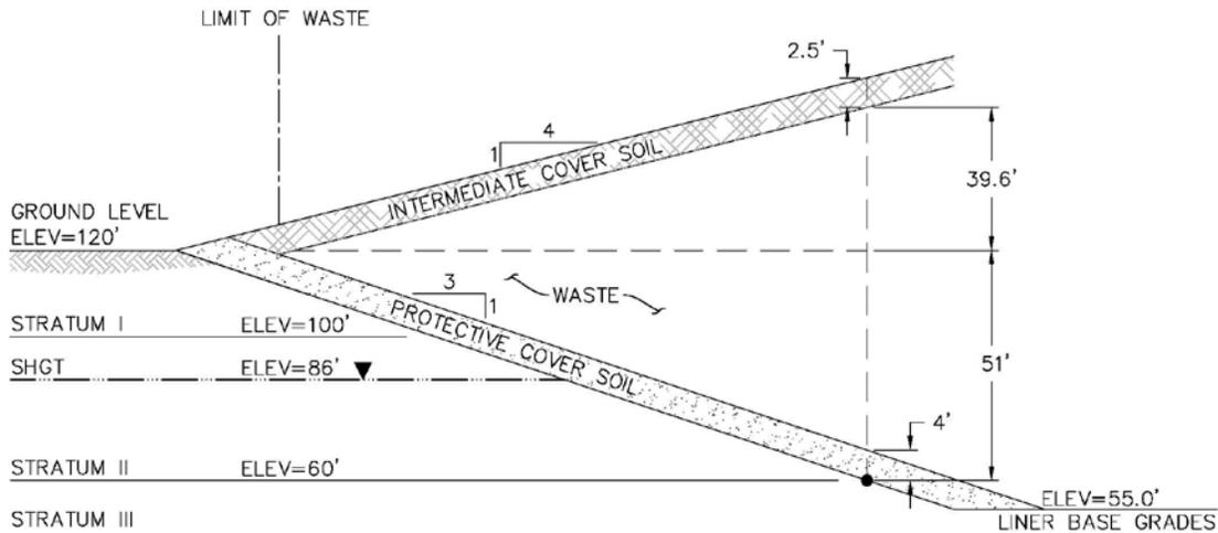
**Figure 3D.4.2-23: Typical/Idealized Cross-Section**
