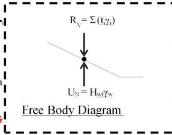
**Body Diagram Layout at Liner Side Slope**
