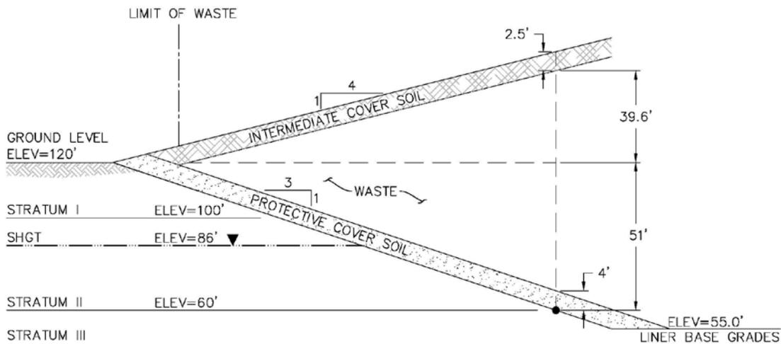
**Figure 3D.4.2-2: Typical/Idealized Cross-Section**
