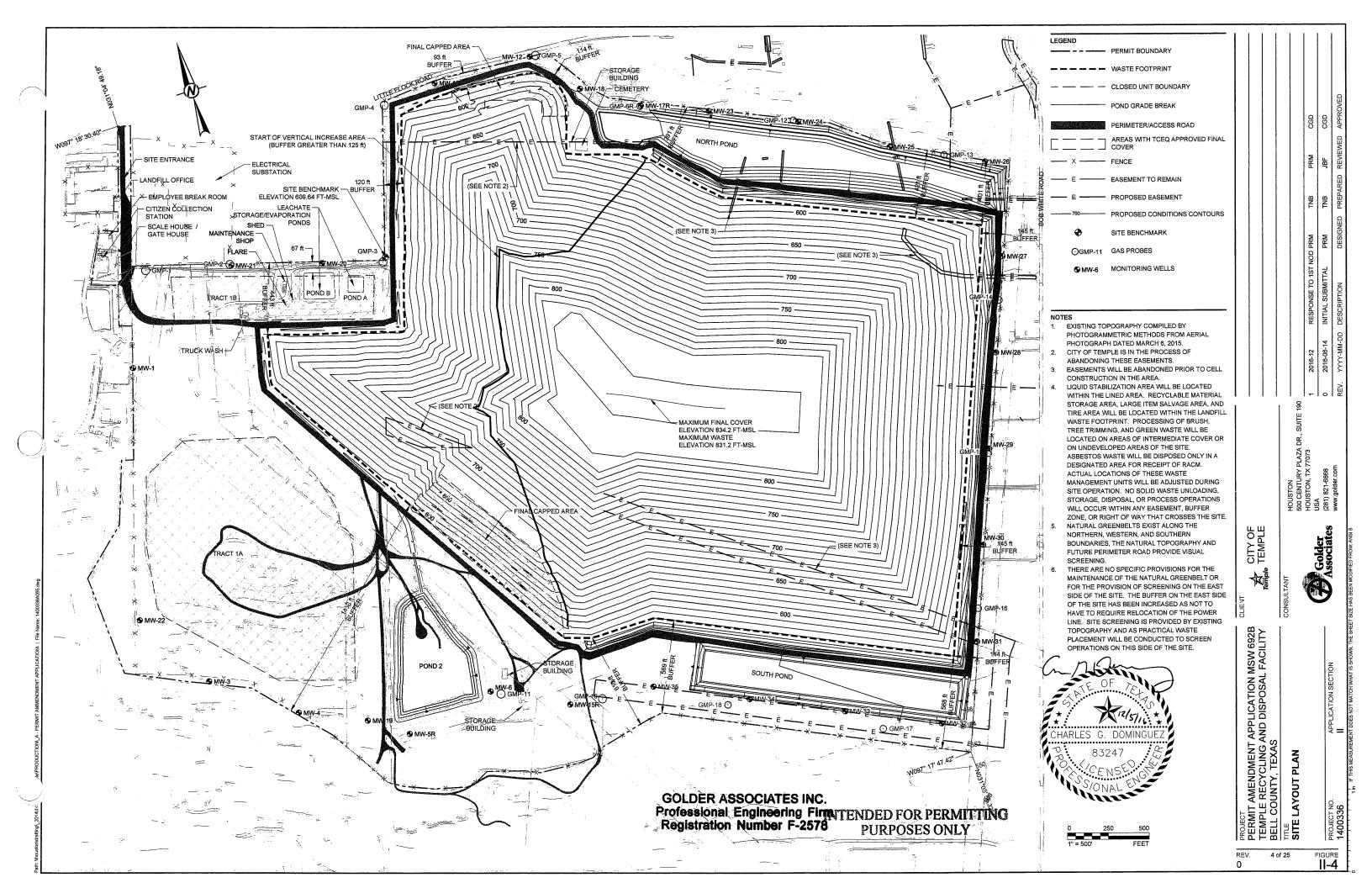
The area outside the waste disposal footprint is used for buffer and landfill facilities, including the gatehouse and scales, landfill access road, leachate storage ponds, leachate force main, and landfill gas flare. As part of the MSW Permit 692A overall development, two detention ponds have been constructed. All surface water from the disposal area is routed through a pond prior to exiting the site.
